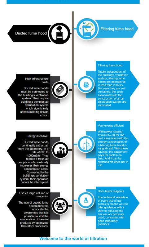
Welcome to the world of innovation, energy saving, ease of operation and environmental protection, where you can get complete protection and a new set of laboratory design
